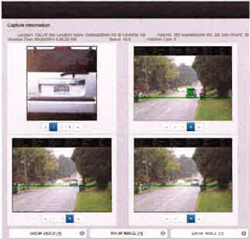
The initial review screen provides the processor with raw images and violation data from which the processor makes the initial determination of whether your violation criteria have been met.
