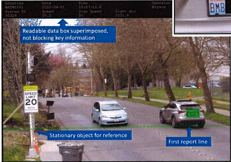
First Image in Color: Vehicle exceeding speed, showing first report line, configurable data box superimposed not blocking info
