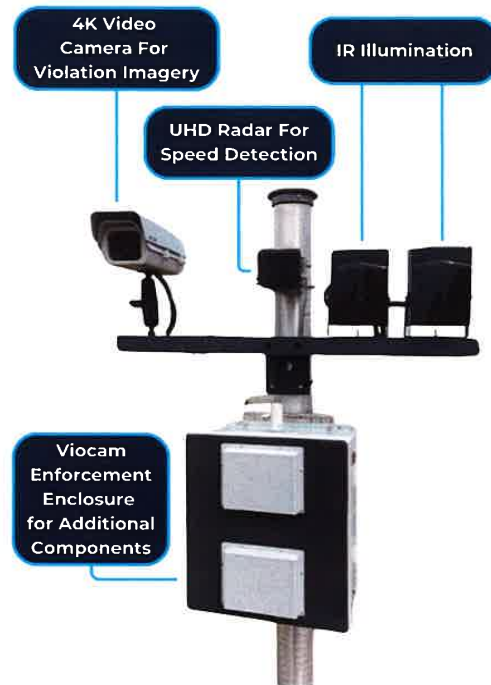
Figure 3: Installed Viocam Vision System for Speed Detection
