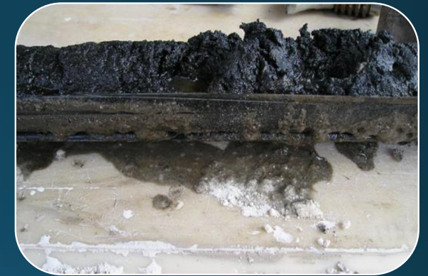
Oily sludge saturated with sulfuric acid PSP-14
